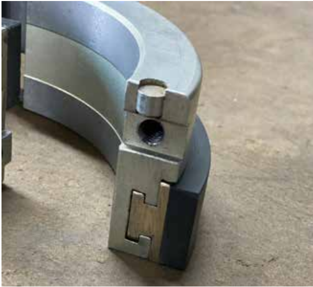
ASSEMBLED FEMALE BAND PRINT SCORER
