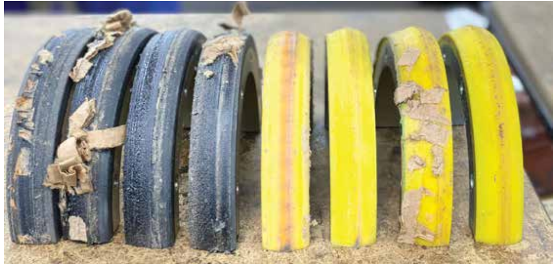
USED CREASING RINGS SENT IN FOR RECOVER
