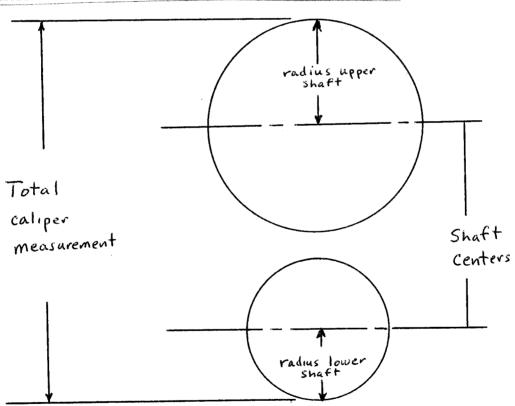
To insure accuracy, measurements should be taken at each end of the shafts and near their horizontal centers. Care must be taken to have the calipers square to the shafts and not tilted to a diagonal. It can be helpful to use the side of a collar to align the calipers. (It is imperative to describe the position of the shafts with each measurement provided. Examples are, shafts maximum open, minimum open, heads tangent, optimum scoring pressure etc.)
