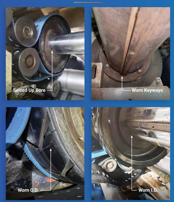
OEM non-split pulleys require a significant downtime event to replace, and interim failures can cause issues with belt tracking and folding rail alignment.
